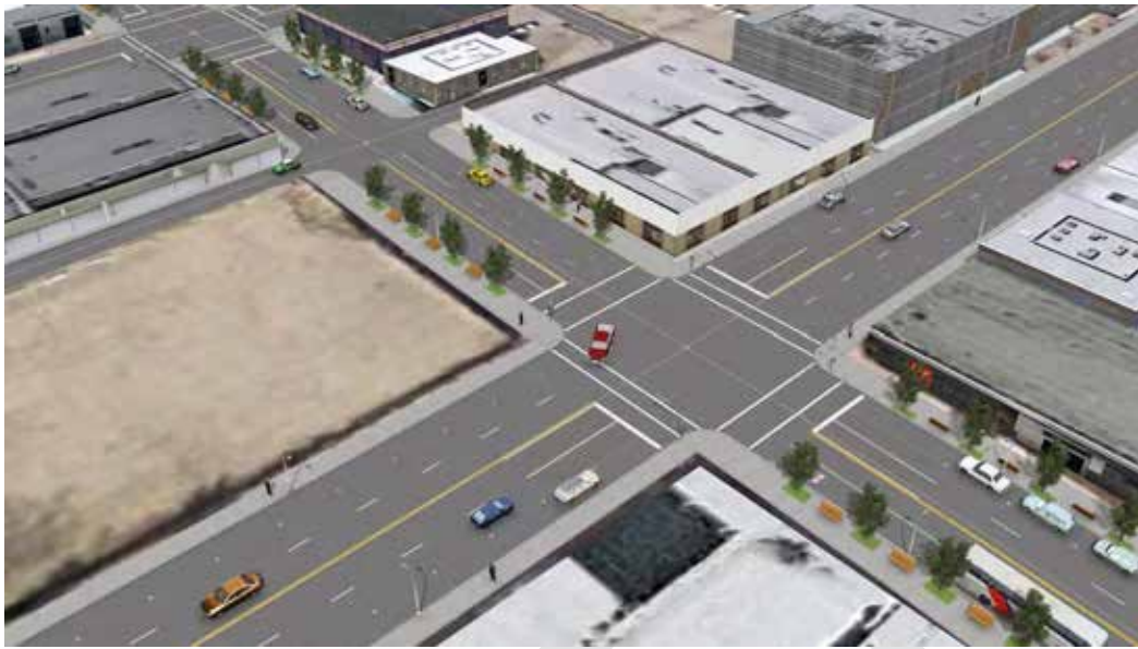
Figure 4-4: Parking Scenario 2a – Parallel Parking on the East Side Only and Sidewalk Widening
